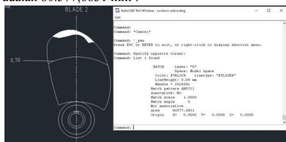
Gambar 7. Luas area repair blade 2
