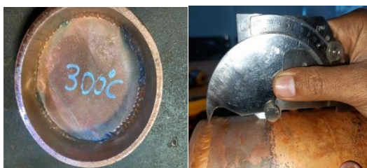
Gambar 5. Visual Test preheat 350°C
