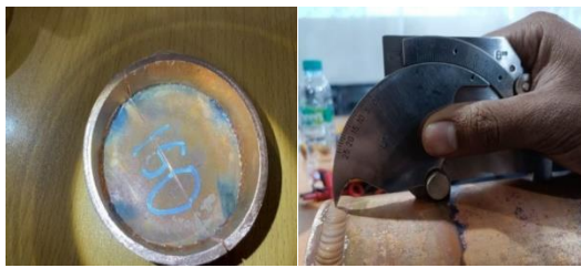
Gambar 3. Visual test preheat 150°C
