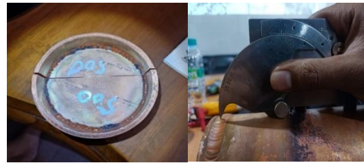
Gambar 6. Visual Test preheat 500°C
