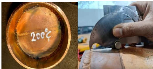
Gambar 4. Visual Test preheat 200°C
