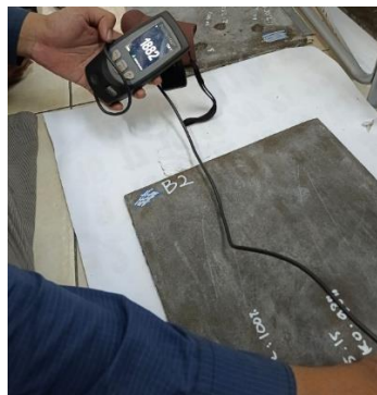
Gambar 3. Pengujian Dry Film Thickness
