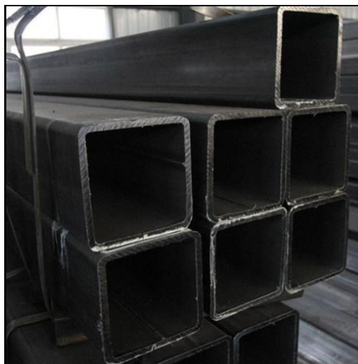
Gambar 1. Material Square pipe ST 37
