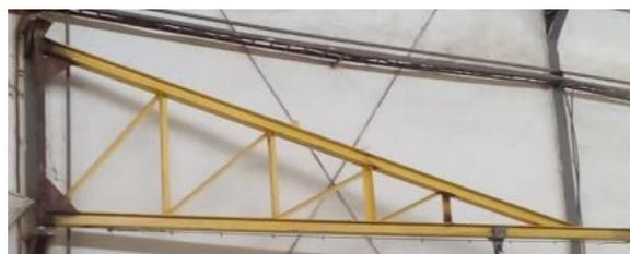
Gambar 1. *Wall jib crane SWL 5 ton*
