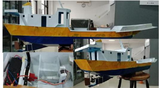
Gambar 9 Model uji free running model test
