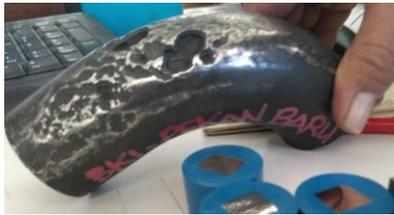
Gambar 1. Tube end bocor
