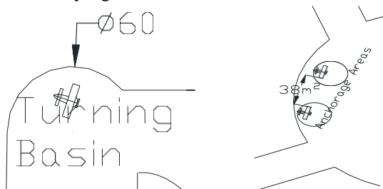
Gambar 23 Turning Basin Gambar 24 Anchorage Areas
