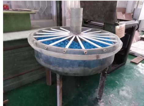
Gambar 5. Desain Unit Clearator Portable
