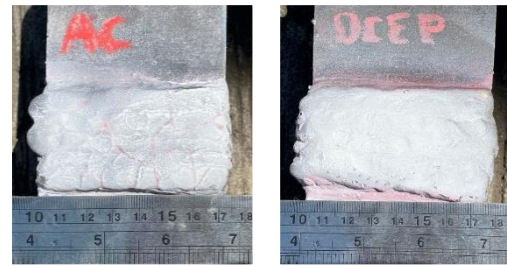
Gambar 2. Hasil Uji Liquid Penetrant
