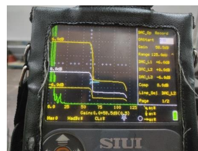
Gambar 3.9 Kurva DAC 20 mm Interpass temperature 450 °C
