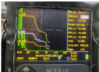
Gambar 4.2 Kurva DAC 10 mm Interpass temperature 150 °C
