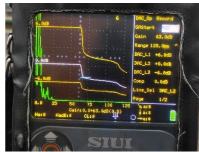
Gambar 3.3 Kurva DAC 10 mm Interpass temperature 150 °C
