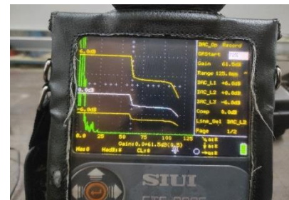
Gambar 3.8 Kurva DAC 10 mm Interpass temperature 150 °C
