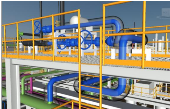
Gambar 1. Naviswork Layout Design of Venting Control Valve1 (Pribadi, 2018)
