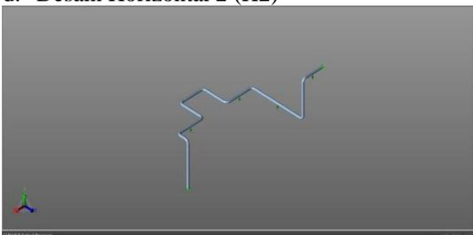
Pada desain HH2 didapatkan nilai tegangan manual *Thermal load* 41001,3 Kpa, *Occasional load* 1397,3 Kpa & *Sustain load* 664,4 Kpa. Pada *Software Thermal load* 50255,4 Kpa, *Occasional load* 2865,2 Kpa & *Sustain load* 9644,4 Kpa. Nilai *pressure drop* manual 0,00041 bar & *software PIPE FLOW EXPERT* 0,0002 bar.
