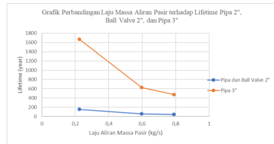
Gambar 3. Lifetime Pipa 2'', Ball valve 2'', dan Pipa 3"
