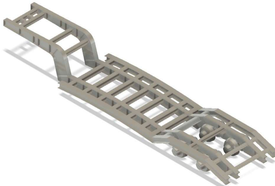
Gambar 4. 3D Modeling Lowbed Trailer
