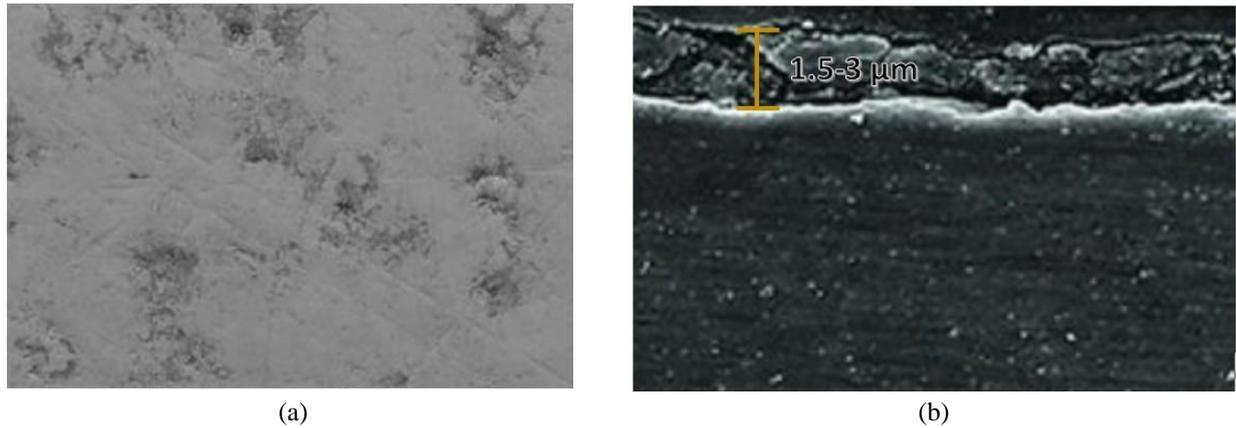
**Figure 4.** Pre-anodized (left) and Anodized (right) sample conducted microhardness test
