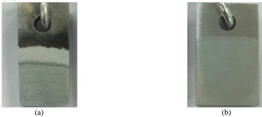
**Figure 1.** aluminum substrate coated sample by (a) Anodization, (b) PEO coating,
