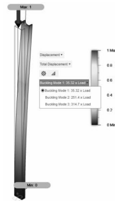
Gambar 5. Analisis Buckling Struktur Utama Redesign Product
