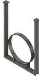
Gambar 6. Resting support with clamp
