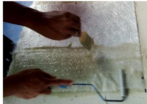
Gambar 1. Proses hand lay up
