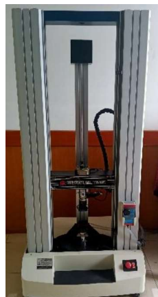
Gambar 5. Universal testing machine
