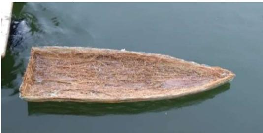
Gambar 3. Hasil cetakan *Natural Fiber Reinforced Boat*
