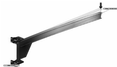
Gambar 10. Nilai defleksi wall jib crane ASTM A515
