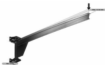
Gambar 7. Nilai defleksi wall jib crane
