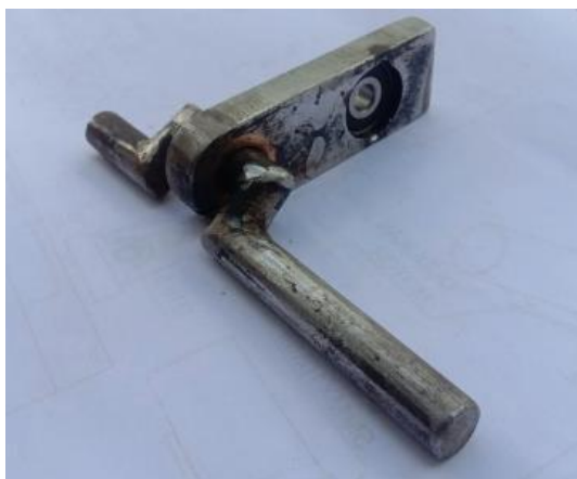
Gambar 3. 6 Sistem Transmisi Crankshaft
